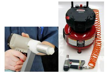
**Figure 1.** Photo of the Zephyr-E equipment in the fired position with bolt head protruding (left) and the unfired position attached to a standard air compressor (right). See online version for figure in color.
